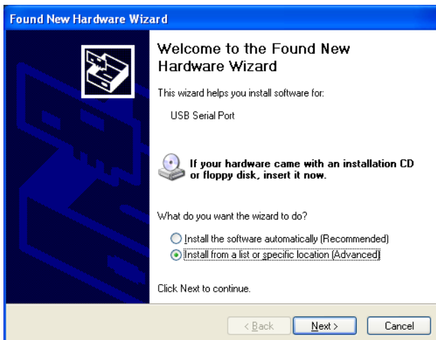
Figure 1: Found New Hardware Wizard with option to install drivers from a specific folder
